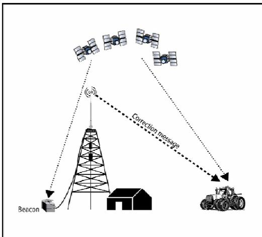
The vehicle (rover) with a GPS antenna receives GPS signals from the GPS satellite constellation. The Beacon receiver, at a known location, receives GPS signals. The beacon generates an equation that changes the location of where the GPS satellites *indicate* it is, to where it *knows* it is, and then sends the equation, known as the “correction message,” to the GPS antenna on the rover—which then applies the correction.
